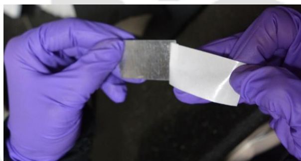
Figure A5.6 Physical abrasion of the developed fingerprint substrate using a double sided tape.
