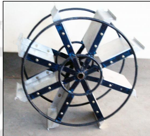
Figure 4.20 (b): Radial paddle wheel is suitable for low speed sail boat.
