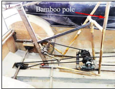
(d): Experimental prototype making of the Cross Trainer mechanism by bamboo.
