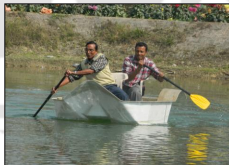
(b): Stability test in water with catamaran type hull.
