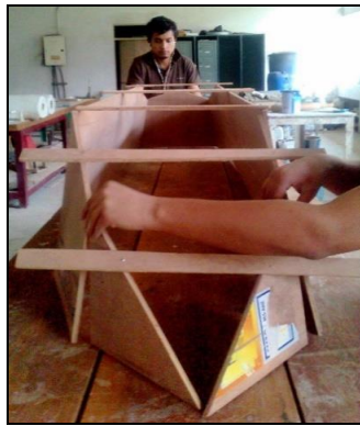
(a): Fabrication of the catamaran hull (front view).
