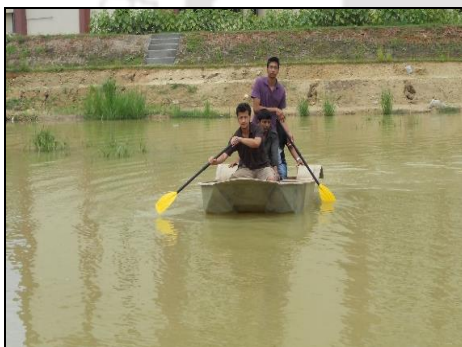
(a): Stability test in water using wooden pattern with three persons.
