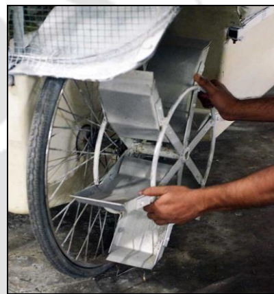
(b): Removing paddle wheel from the wheel shaft with anti-clockwise rotation.
