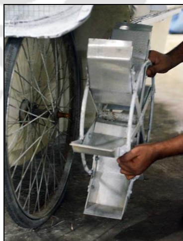
(c): Removing the paddle wheel from the wheel shaft.
