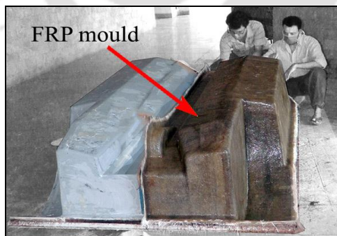
Figure 4.5 (c): Preparation of FRP mould using the pattern.
