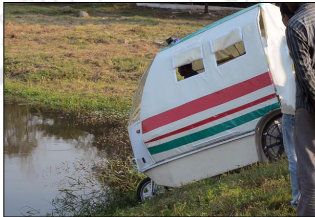
(a): Trial of modified version of functional prototype in water.
