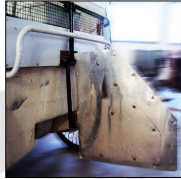
(b): Modified rudder after field trial.
