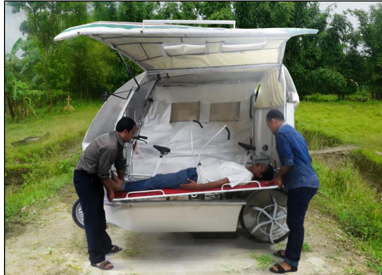
Figure 5.2: Test for loading and unloading the patient with stretcher in the ambulance. Source of Photographs: Author
