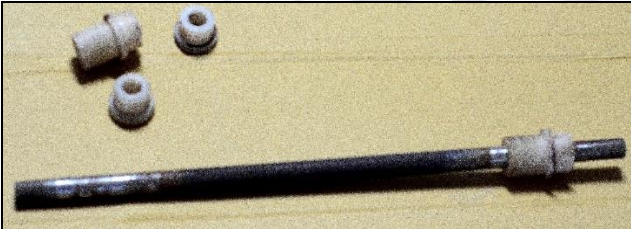
(c): Shaft of the handlebar with sleeve.
