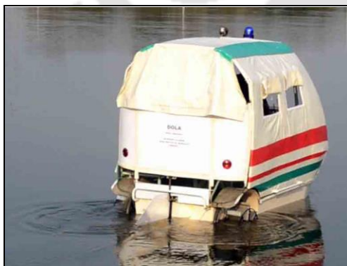
(a): When rudder moves left direction, amphibian turns right direction.
