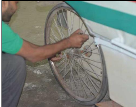
(b): Removing rear wheel from the wheel shaft with anti-clock wise.
