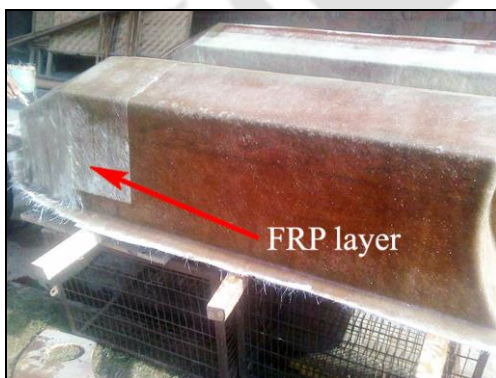
(f): Application of one layer of FRP on the wooden pattern to strengthen.
