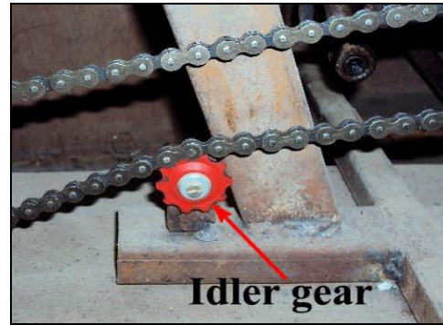
(b): Idler gear placed between rear free wheel gear and intermediate shaft.
