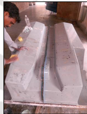
Figure 4.5 (b): Smoothing the surface of the pattern for applying releasing agent.
