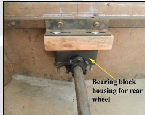
(b): Details of bearing block housing mount on the chassis.
