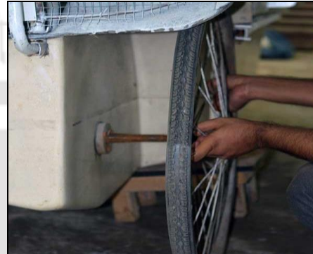
(c): Removing the rear wheel from the wheel shaft.
