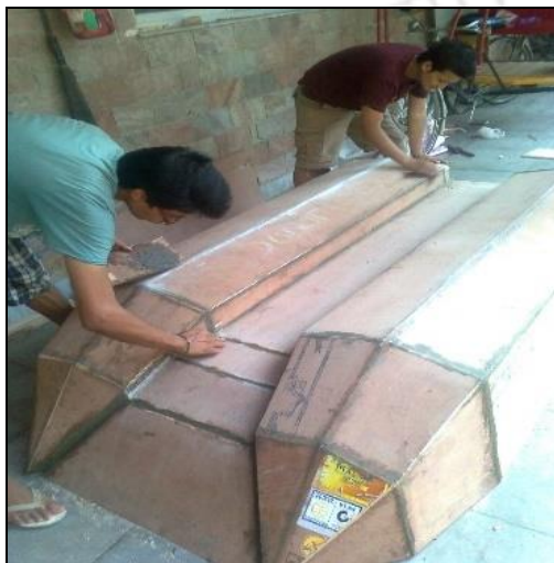
(d): Preparation of pattern for catamaran type hull; applying FRP putty.
