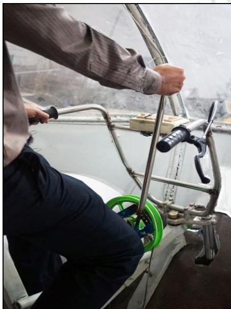
(a): Steering pilot drive (green coloured wheel) on the pedestal head.
