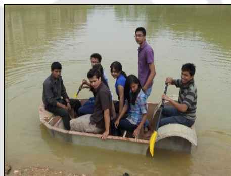
(b): Stability test in water using wooden pattern with the maximum flotation.
