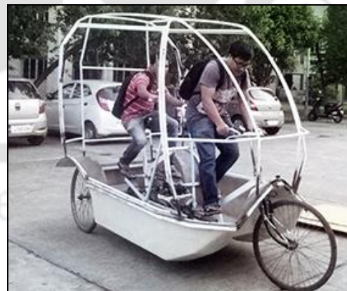
(d): The front wheel fork was broken while being used by two persons in the second time.
