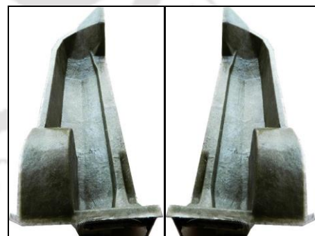
Figure 4.5 (d): FRP split mould after release from the pattern.
