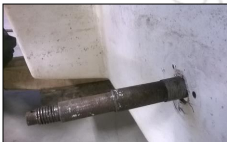
(c): Rear wheel shaft before fixing the oil seal.
