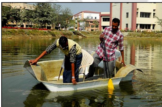
(a): Trial in water with FRP catamaran type hull.
