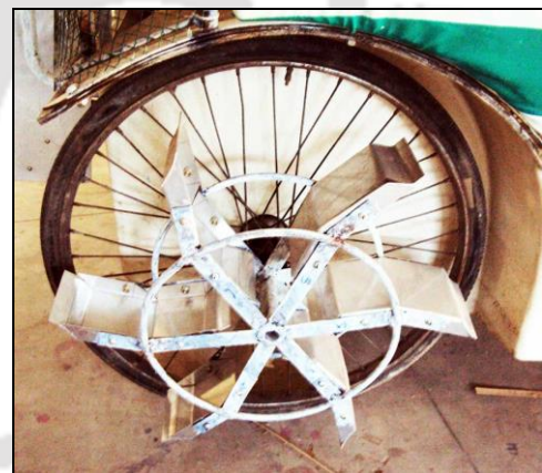
(d): Feathering paddle wheel design with angular paddle.
