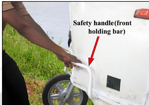
(b): A Safety handle is used for holding and pulling the vehicle when it gets stuck in muddy water.
