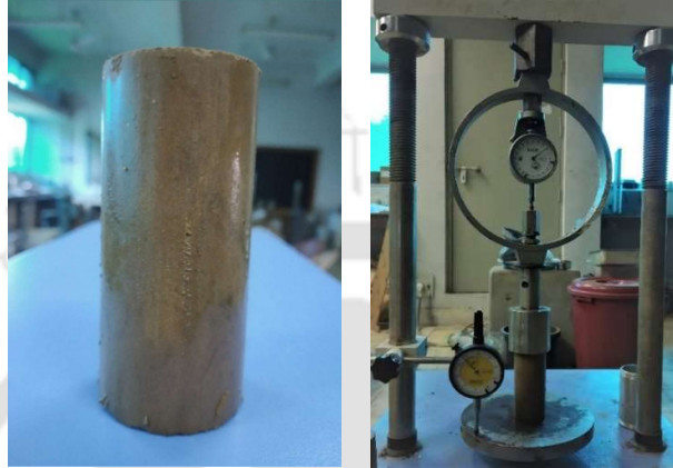
Fig. 3.13 Sample preparation and apparatus for UCS test
