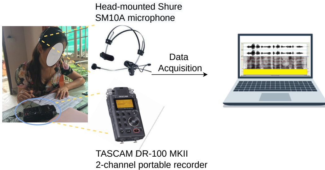
Figure 3-2: Demonstrating the overall setup for recording the Changki Mongsen Chungli-Ao (CMC-Ao) Corpora.
