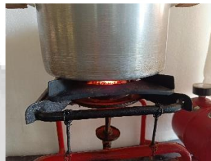
Figure 5.8 Pictorial representation of no soot formation in PMC based ethanol cookstove
