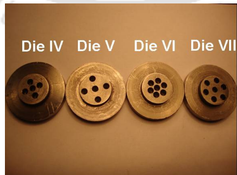
Figure 3.13. Four types of dies used to study the effect of die pocket
