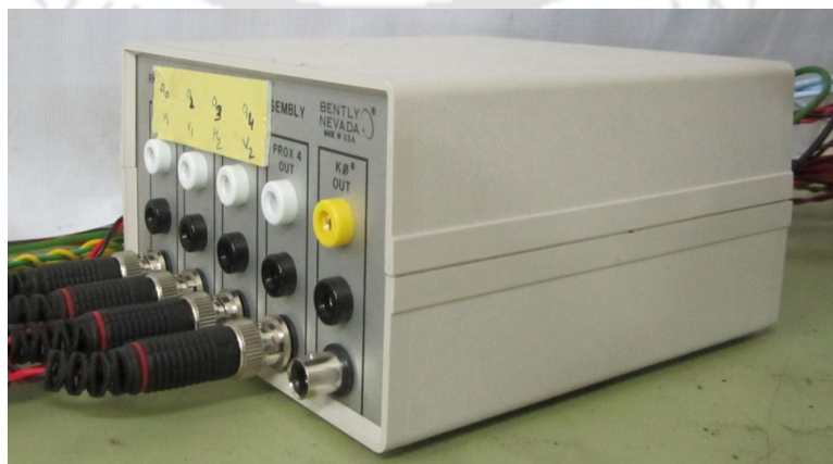
Figure 5.11 A proximity amplifier with four channels
