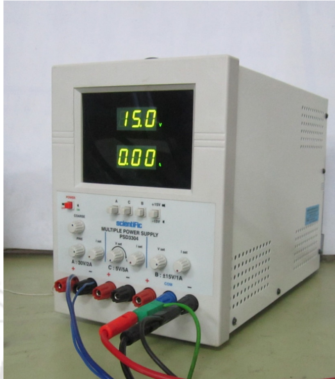
Figure 5.12 A constant DC power source
