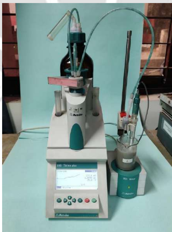
Fig. 3.6 Photograph of automatic potentiometric titrator during the test
