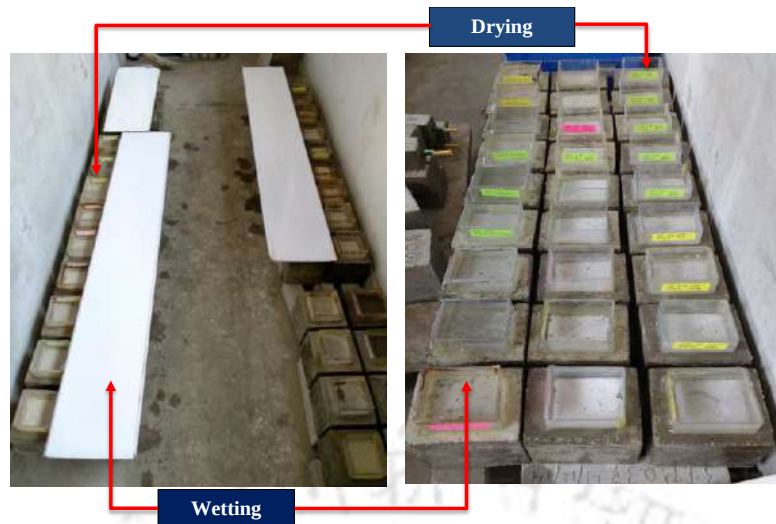
Fig. 3.15. Photograph of cube specimens subjected to alternating wetting-drying cycles
