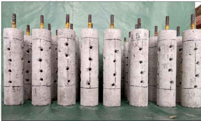
Fig. 3.12 Photograph of the drilled cylindrical reinforced concrete specimens
