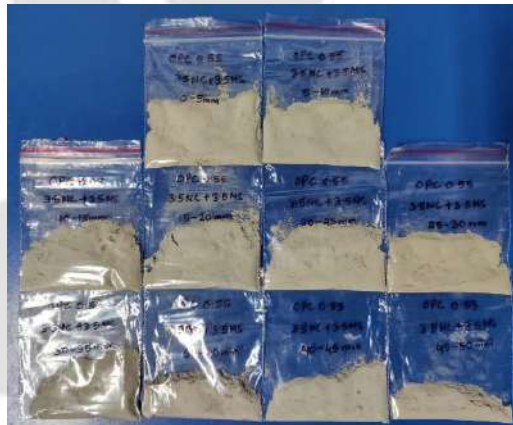
Fig. 3.17 Photograph of concrete powder samples obtained from different depth intervals
