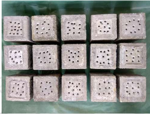
Fig. 3.16 Photograph of drilled concrete specimens
