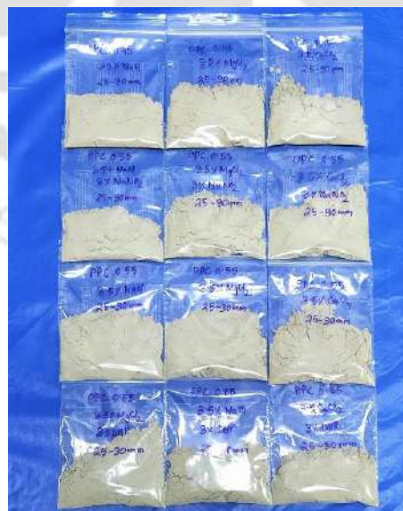
Fig. 3.13 Photograph of concrete powder samples obtained from the rebar level (25-30 mm) of cylindrical reinforced concrete specimen
