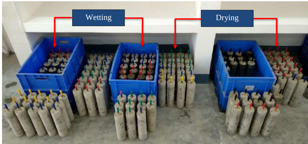
Fig. 3.9 Photograph of cylindrical reinforced concrete specimens subjected to exposure solutions
