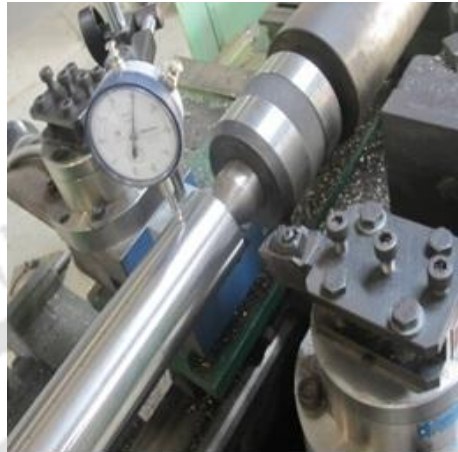
Figure 3.7. Diametral error measurement by dial gauge
