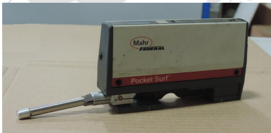
Figure 3.10. Surface roughness measurement by Pocket Surf
