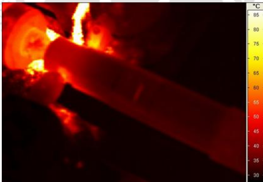
Figure 4.14. Thermogram of mild steel workpiece during cutting (75 m/min cutting speed, 0.08 mm/rev feed, 1 mm depth of cut and 10 mm distance between cutting tools)
