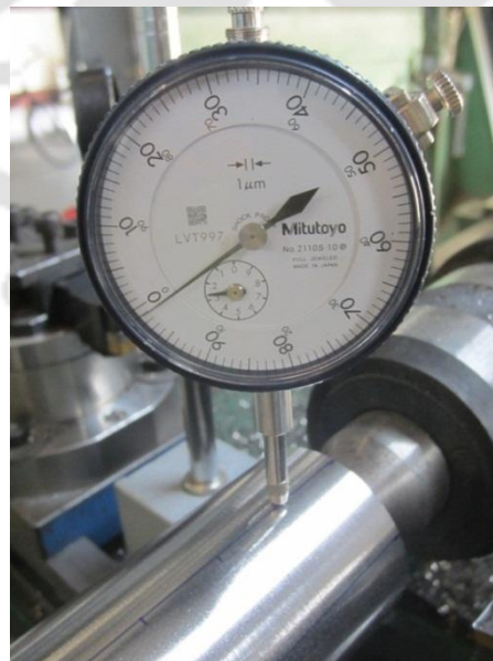
Figure 5.3. Measurement of the diametral error
