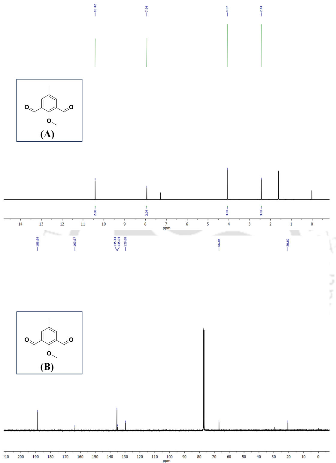
Figure 3.37 ^1\text{H} NMR (A) and ^{13}\text{C} NMR (B) spectra of 2-methoxy-5-methylisophthalaldehyde in the Chloroform- d solvent.
