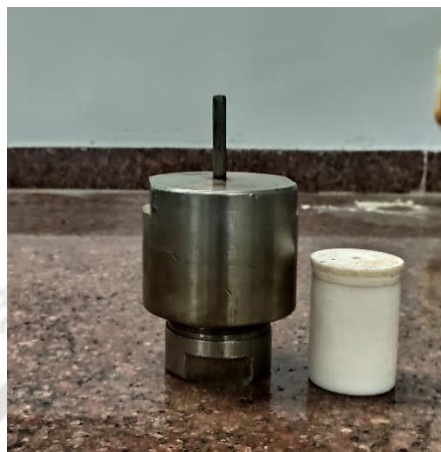
Figure 2.1: Autoclave reactor for MOF and MOF-nanoparticle synthesis
