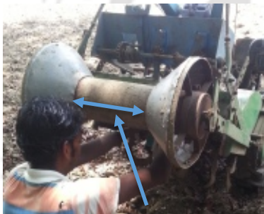
Figure A4.5. The bed shaper cone can be set for different bed sizes.
