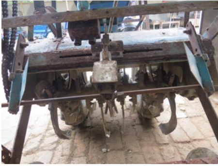
Figure A4. 20. Scrapper fixed to the BP.
