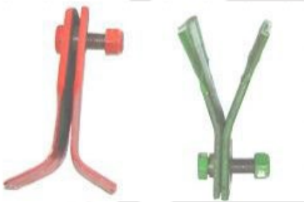
Figure A4.33. J-type and Gamma-type flail blades used in Happy Seeder. Source - (Jat et al., 2013)
