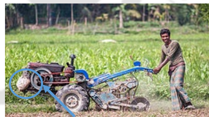
Figure A4.8. Counterweight in the front to ease lifting the BP (Source: CIMMYT).
