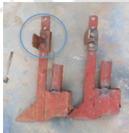
Figure A4.7. The furrow opener can be set anywhere in the given slot.
