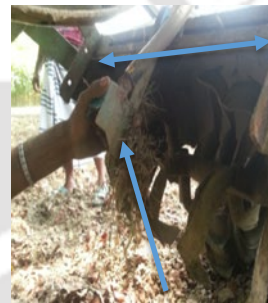
Figure A4.6. Depending on plowing depth, the furrow opener depth hole needs to be selected.
