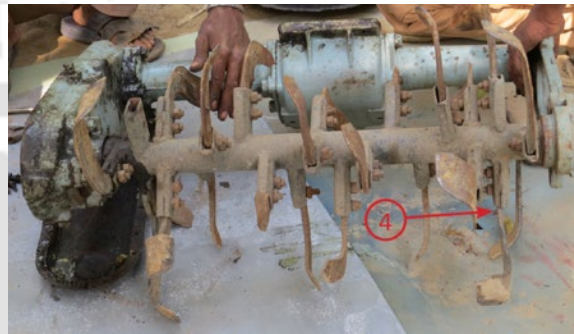
Figure A4. 17. 4: The larger blades tend to bend or break at this point.
