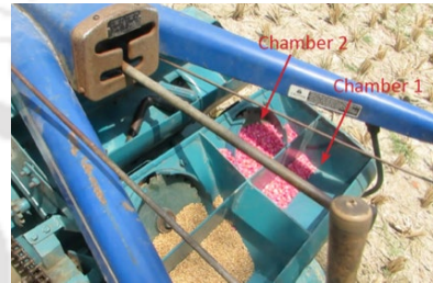
Figure A4. 25. Seed from chamber 1 to 2 is supposed to be manually transferred. Chamber 1 acts as the storage, while chamber 2 is meant for metering and dispensing.
