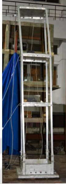
Figure 3.3 Image of damaged shear building at the end of experimental investigation
