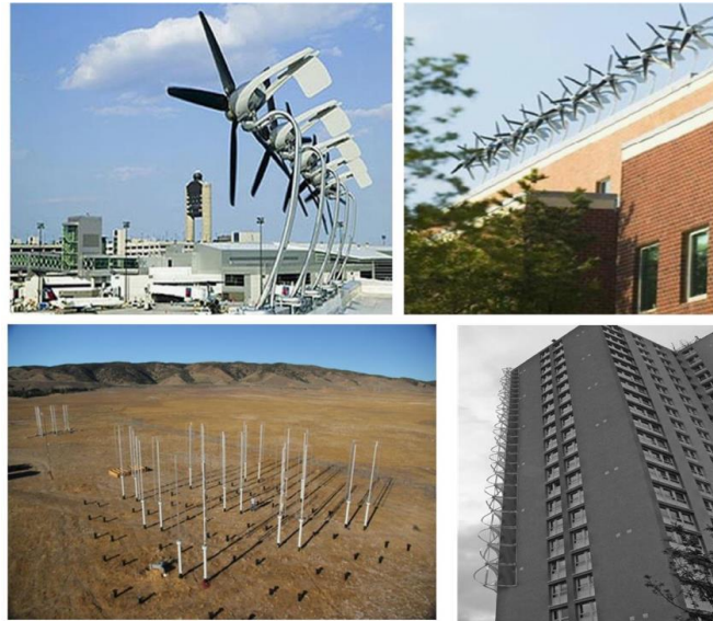
Fig. 2.5 Cluster arrangement of small wind turbine (Liu et al. 2019; Dilimulati et al., 2018; Casini, 2016)
