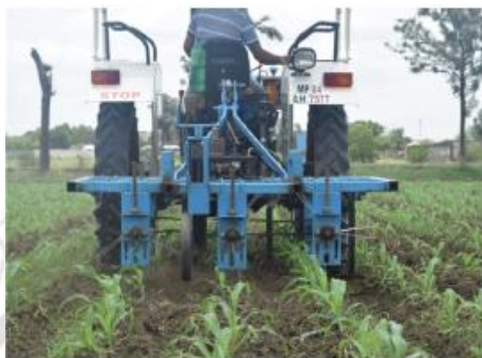
Figure 2.16 Integrated inter and intra-row weeding system (Chandel et al., 2021)
