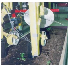
Figure 2.17 Rotating disc tine (Cavalieri et al., 2001)
