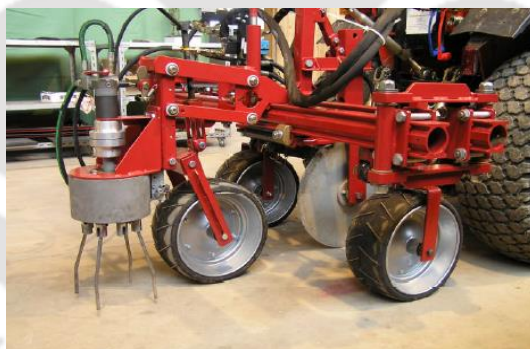
Figure 2.18 The cycloid hoe (Griepentrog et al., 2007)
