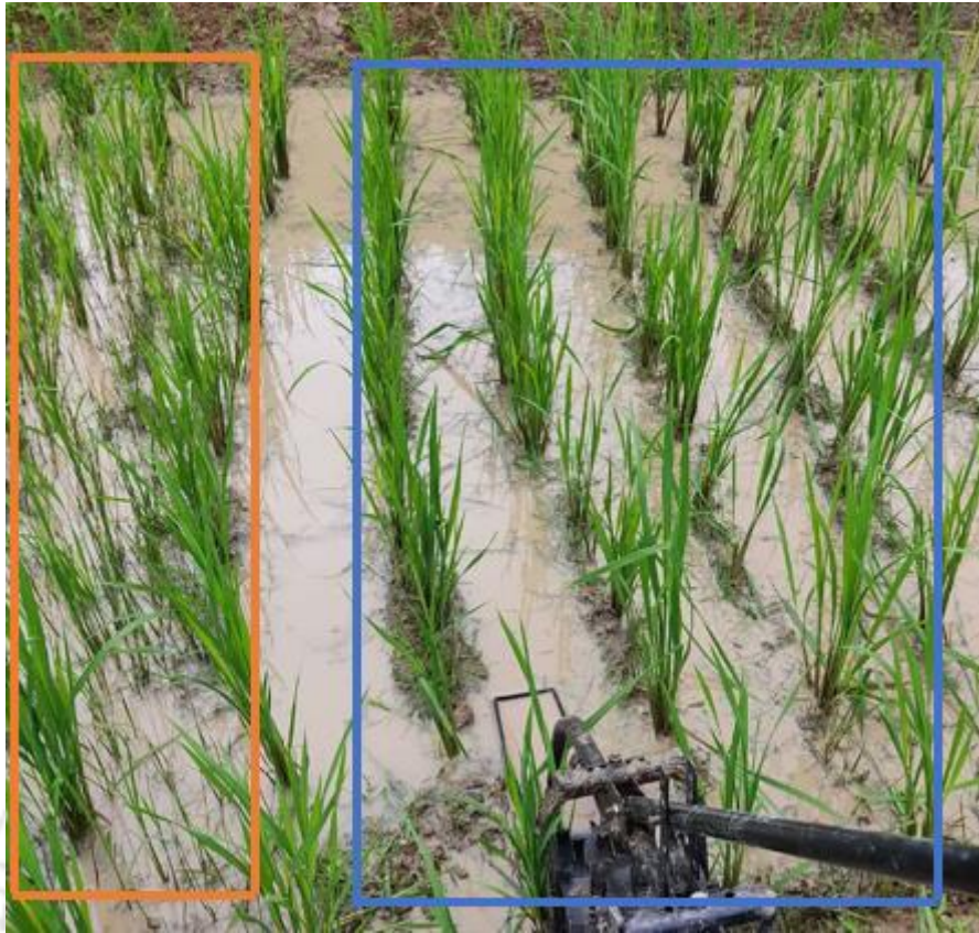
Figure 3.12 Field conditions before and after the operation of the weeder (the area inside the orange boundary indicates the field conditions before the operation of the weeder and the area inside the blue boundary indicates the field conditions after the operation of the weeder)
