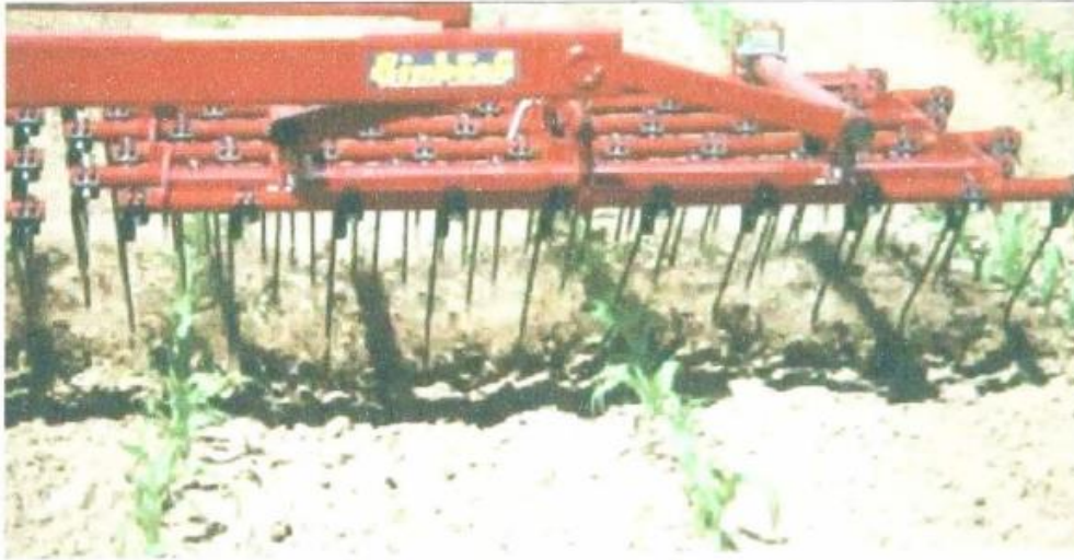
Figure 1.4 Floating spring-tine harrow weeder (Home, 2003)
