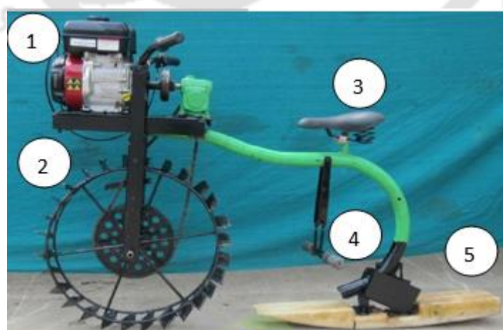
Figure 2.1 A self-propelled ride-on type paddy weeder (Basavaraj et al. 2018)
