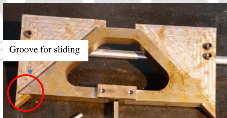
Figure 5.2 Trapezoidal and lateral plates fabricated with sliding grooves
