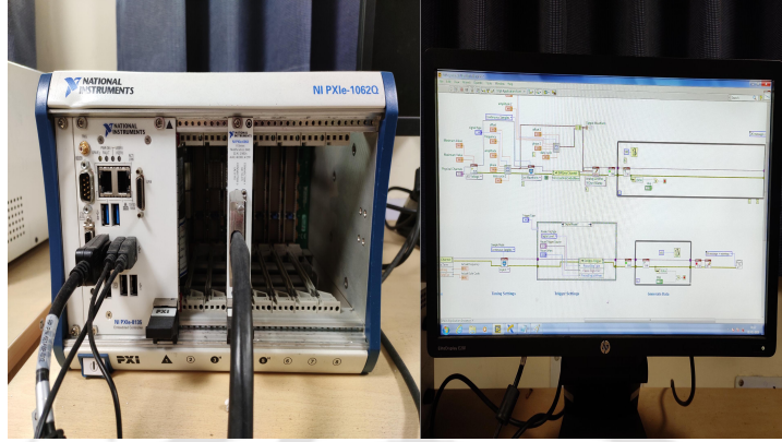
Figure 5.17: PXIE-6363 embedded controller with DAQ module for measuring and storing data
