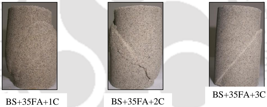
Fig. Patterns of specimens of sand-cement mixes (100 kPa confining pressure) after curing
