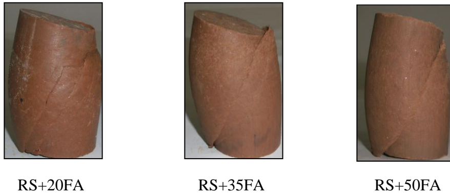
Fig. 8.2(e) Failure patterns of red soil-fly ash specimens \epsilon ring (100 kPa confining pressure)
