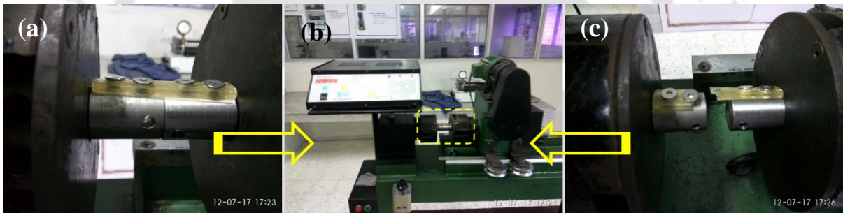
Figure 5.11: Arrangement of bone plates to the torsion machine for torsion testing (a) before fracture (b) arrangement in the machine (c) After fracture.
