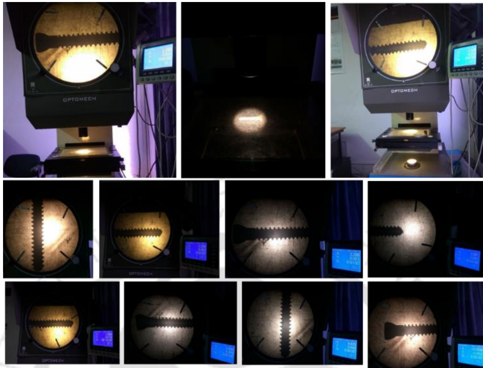
Figure 3.26: Photographic image of surface profile optical micrograph of cortical screws
