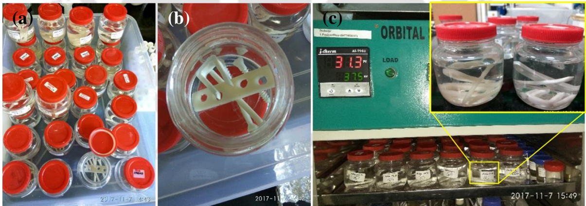
Figure 5.27: Glass jars used for in vitro hydrolytic degradation studies. (b) Magnified view of the bone plate kept in PBS medium (c) arrangement of PBS filled glass jar in hot air oven maintaining the temperature at 37.5°C.
