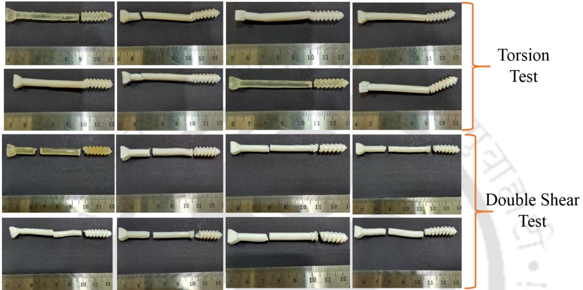
Figure 4.23: Photographic images of fractured cancellous screws after torsion test and double shear strength test.
