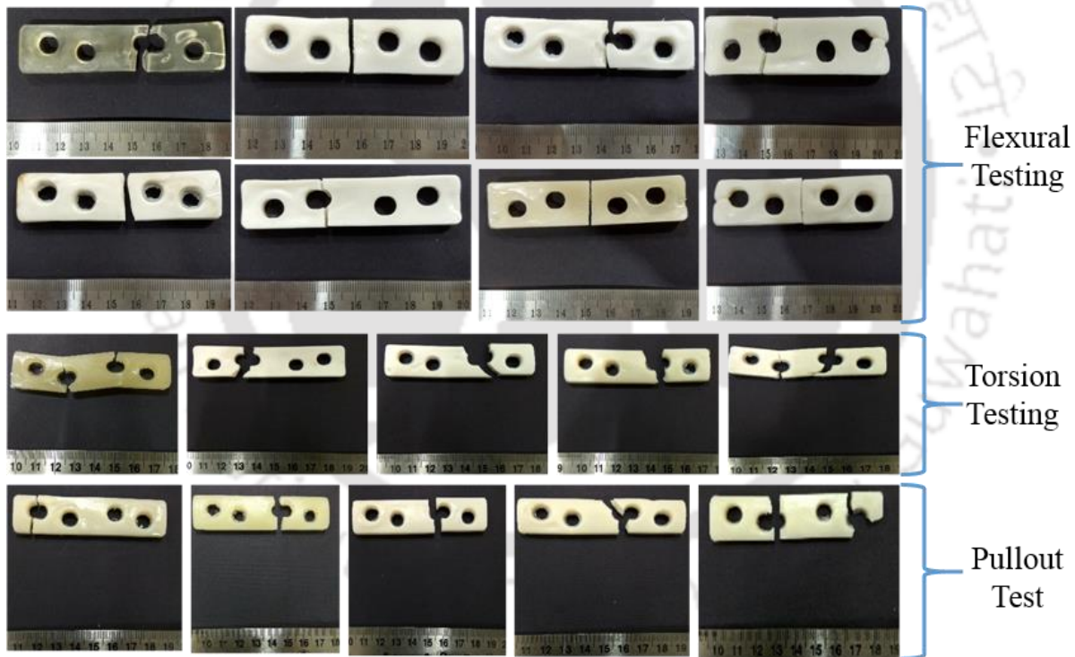
Figure 5.25: Fractured bone plate profile after the mechanical test.
