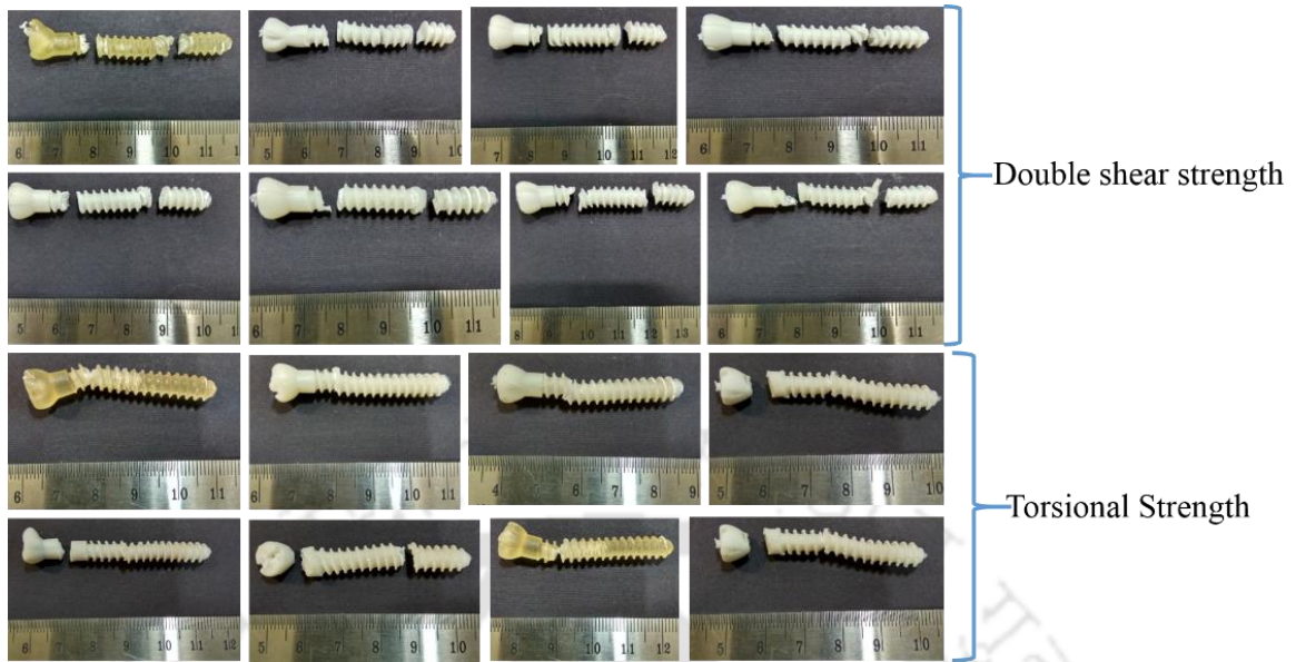
Figure 3.23: Photographic images of fractured cortical screws after double shear strength and torsional strength test.
