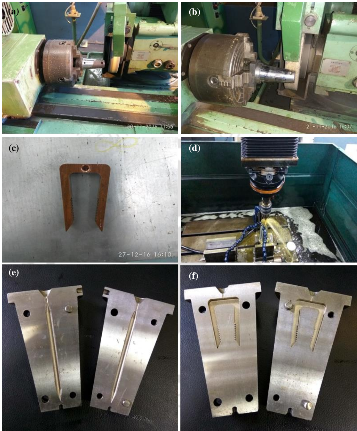
Figure 6.4: Schematic diagrams of pins and staples related to (a) Fabrication of H13 metals in form of mold cavity (b) Machining after heat treatment (c) Bone staples electrode for electric discharge machining (d) Electric discharge machining process (e) Fabricated mold of pins (f) Fabricated molds of bone staples.
