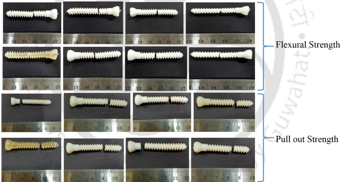
Figure 3.24: Photographic images of fractured cortical screws after flexural test and axial pull-out test.
