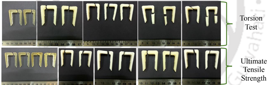
Figure 6.25: Photographic images of Fractured bone staples after torsion and ultimate tensile strength test.
