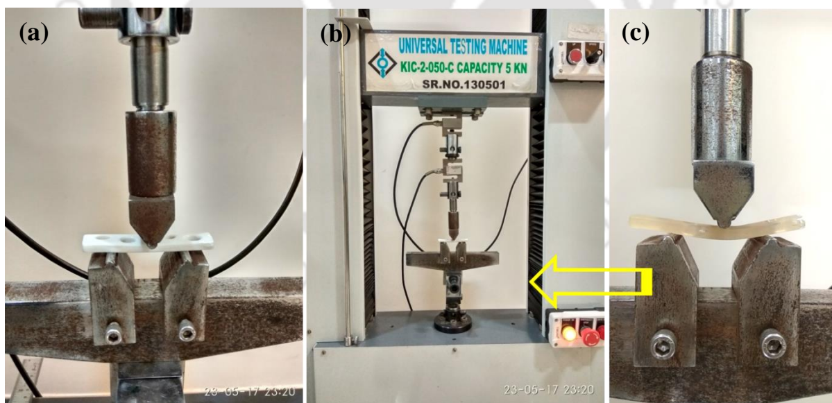
Figure 5.8: Arrangement of 3 point bend test performed on bone plates.
