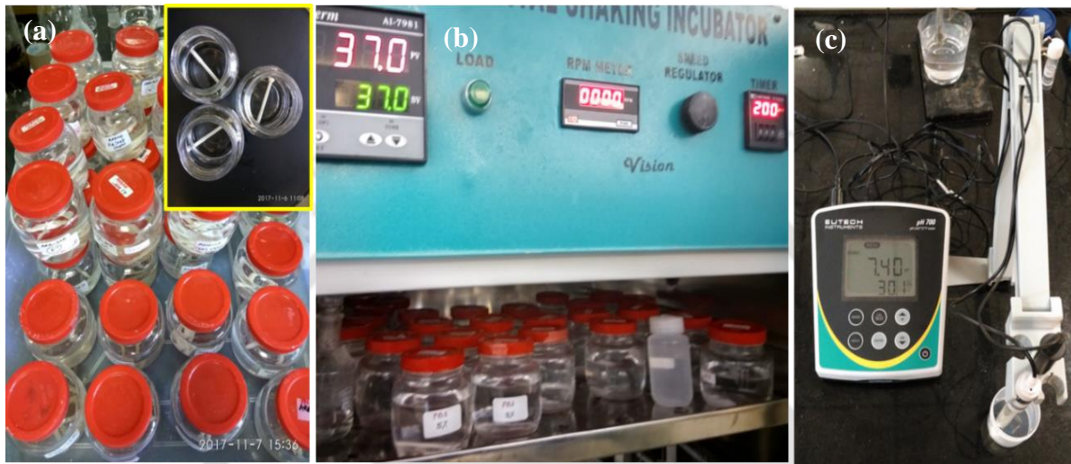
Figure 4.19: (a) In vitro hydrolytic degradation of cancellous screw arrangement in a glass jar (b) Hot air oven maintained at 37° C (c) pH measurement of PBS solution for maintaining the pH routinely.
