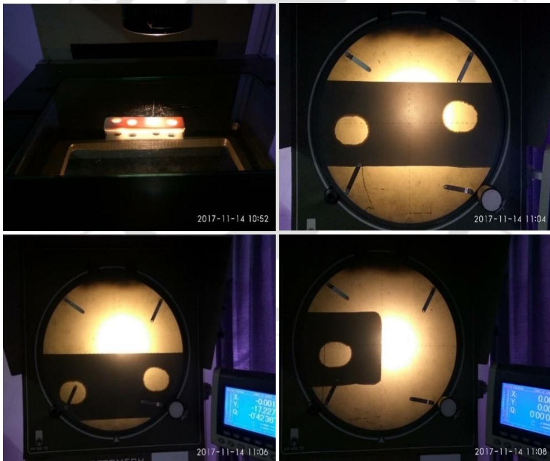
Figure 5.31: Photographic image of surface profile optical micrograph of bone plates.
