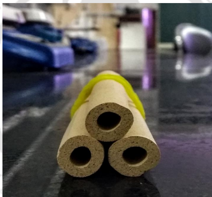
Fig. 3.3 Deformed shaped membrane with 1 wt.% Na-CMC solution
