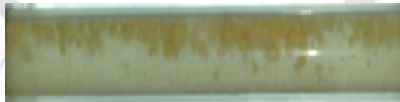
Fig. 4.1f Dispersion of oil in water ( U_{SO}=0.188\text{m/s} ; U_{SW}=0.8\text{ m/s} ).
