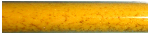
Fig. 4.1g Dispersion of water in oil ( U_{SO}=1.1\text{m/s} ; U_{SW}=0.4\text{m/s} ).
