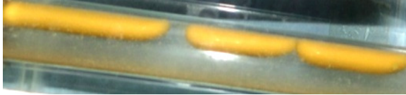
Fig. 4.3b Slug flow ( U_{SO}=0.046\text{m/s} ; U_{SW}=0.169\text{ m/s} )
