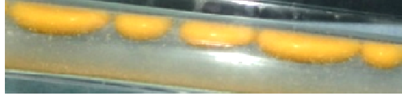
Fig. 4.3a Plug flow ( U_{SO}=0.042\text{m/s} ; U_{SW}=0.169\text{ m/s} )
