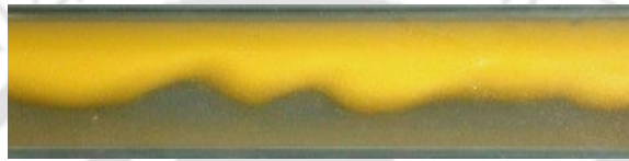
Fig. 4.1c Wavy stratified flow ( U_{SO}=0.103\text{m/s} ; U_{SW}=0.267\text{m/s} ).
