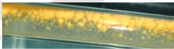
Fig. 4.3f Dispersion of oil in water ( U_{SO}=0.6\text{m/s} ; U_{SW}=0.65\text{ m/s} )
