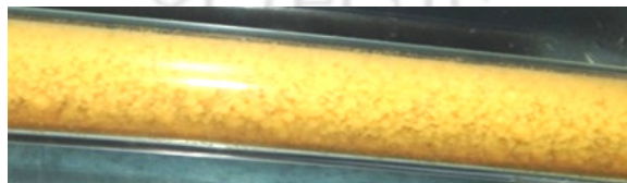
Fig. 4.3g Dispersion of water in oil ( U_{SO}=0.82\text{m/s} ; U_{SW}=0.24\text{ m/s} )
