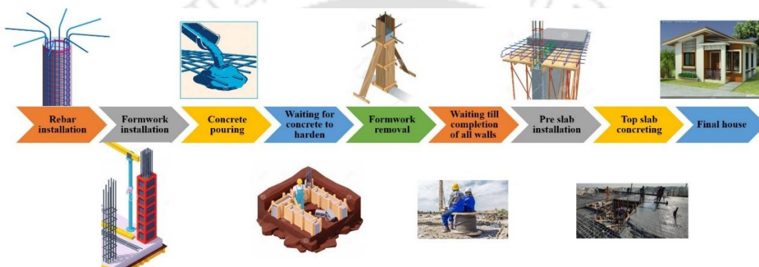
Figure 2.1 Steps in conventional construction method.
