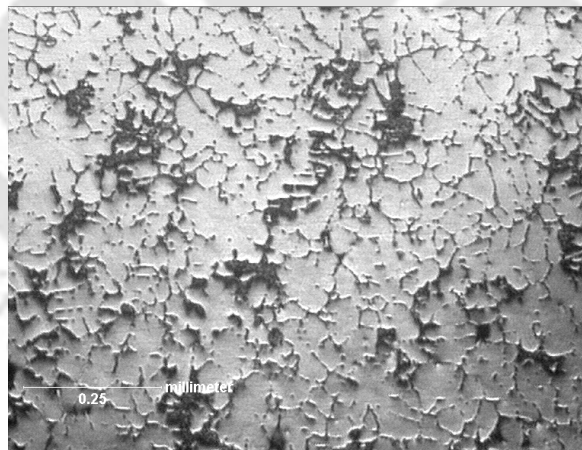
Fig.4.74. Optical micrograph of Alloy- F in undeformed condition
