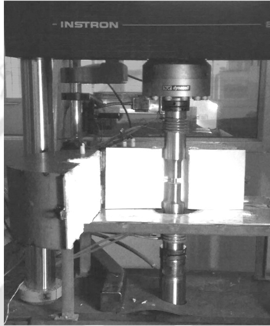
Fig.3.4. The high temperature compression testing set-up
