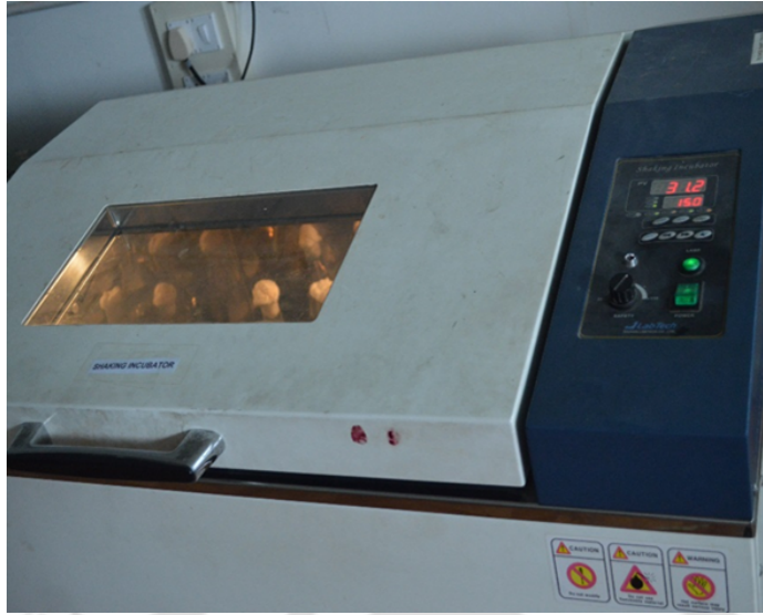
Figure 3.8: Biosorption study in a shaking incubator to maintain optimum conditions
