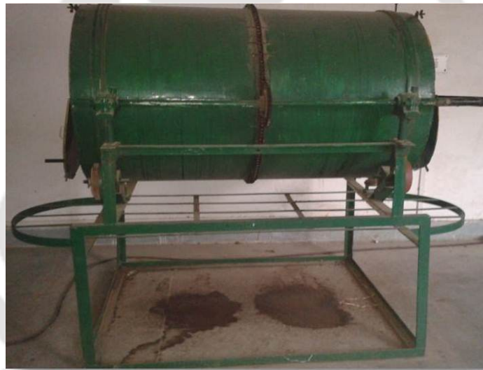
Figure 3.3: Pilot Scale Rotary Drum Composter (a) Schematic design (b) Pictorial view
