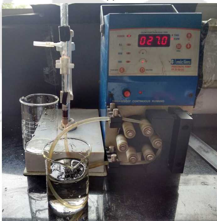
Figure 3.11: (a) Schematic diagram of column setup (b) Pictorial view of column setup
