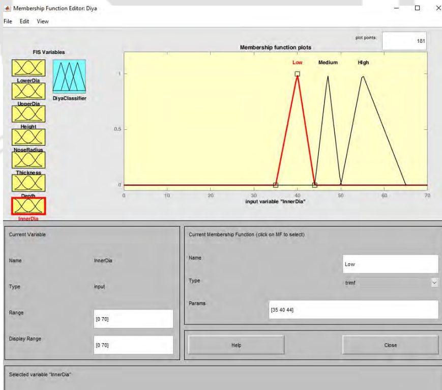
Fig 4.13: Membership function for inner thickness input parameter
