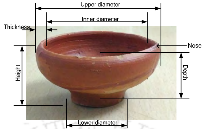
Fig.4.2: Different parameters of a typical Diya (Source: Author generated)
