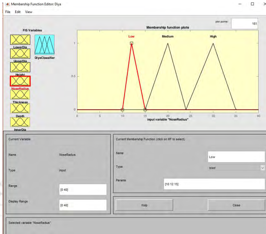
Fig 4.10: Membership function for Nose radius input parameter
