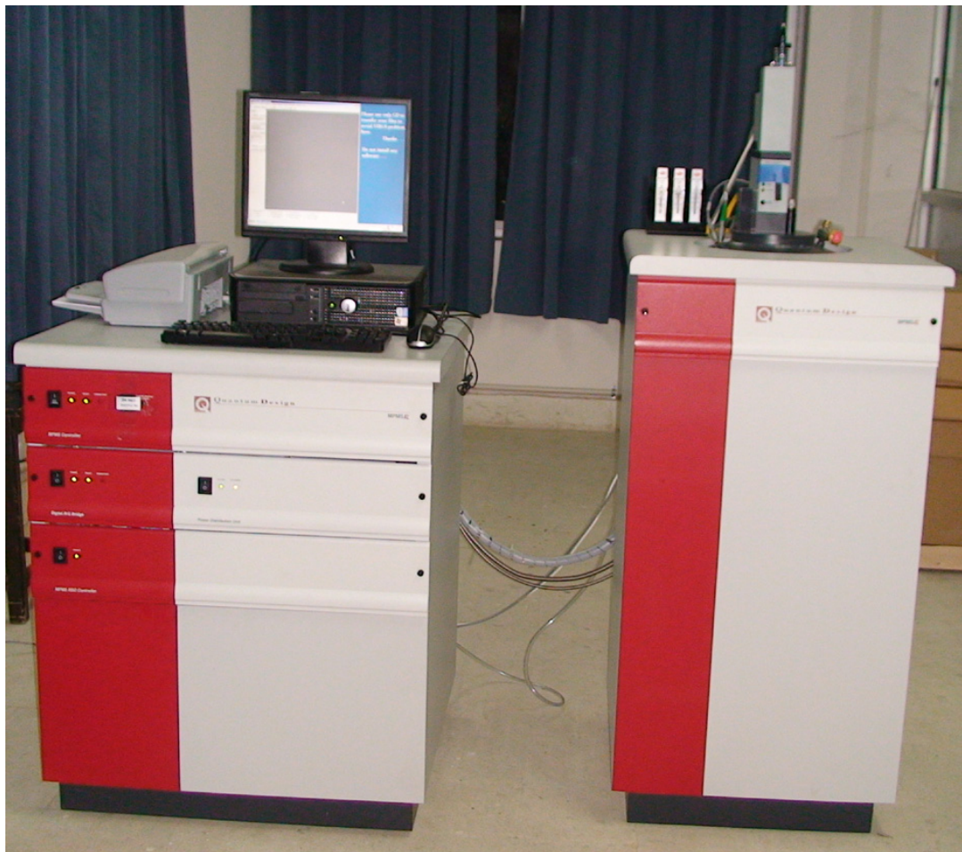
Figure 3.15: Photographic view of a SQUID magnetometer in MPMS (MPMS XL 7 system).
