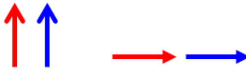
Figure 2.19: Schematic drawing of broadside and head-to-tail configurations for a pair of ferromagnetically coupled magnetic moments.
