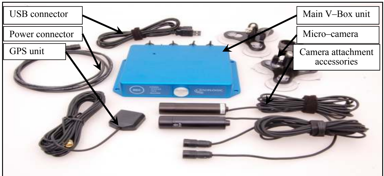
Figure 3.3 The V-Box with its accessories
