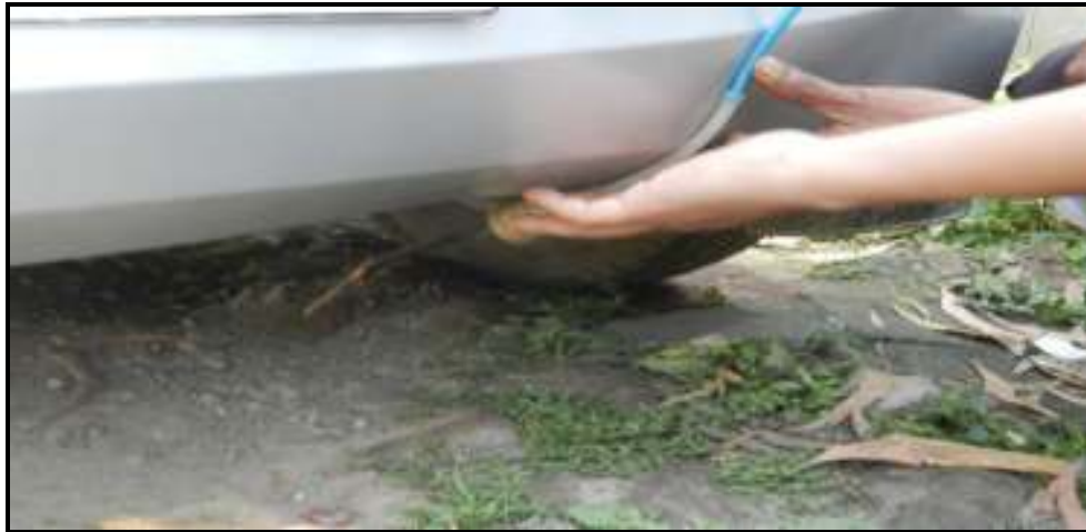
Figure 3.4 Auto-gas analyser probe connection to tail-pipe of a test vehicle
