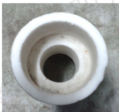
(a) Mixing chamber
