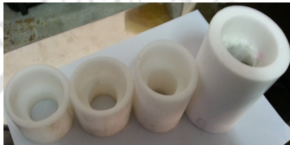
Fig. 4.14. Different types of mixing chambers
