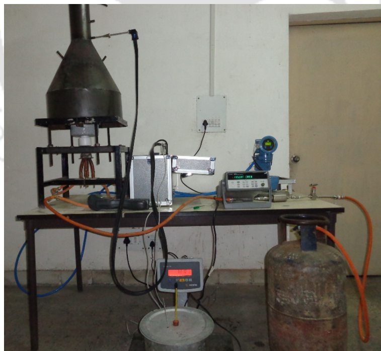
Fig. 5.8. Pictorial view of the experimental set up- for measuring emissions
