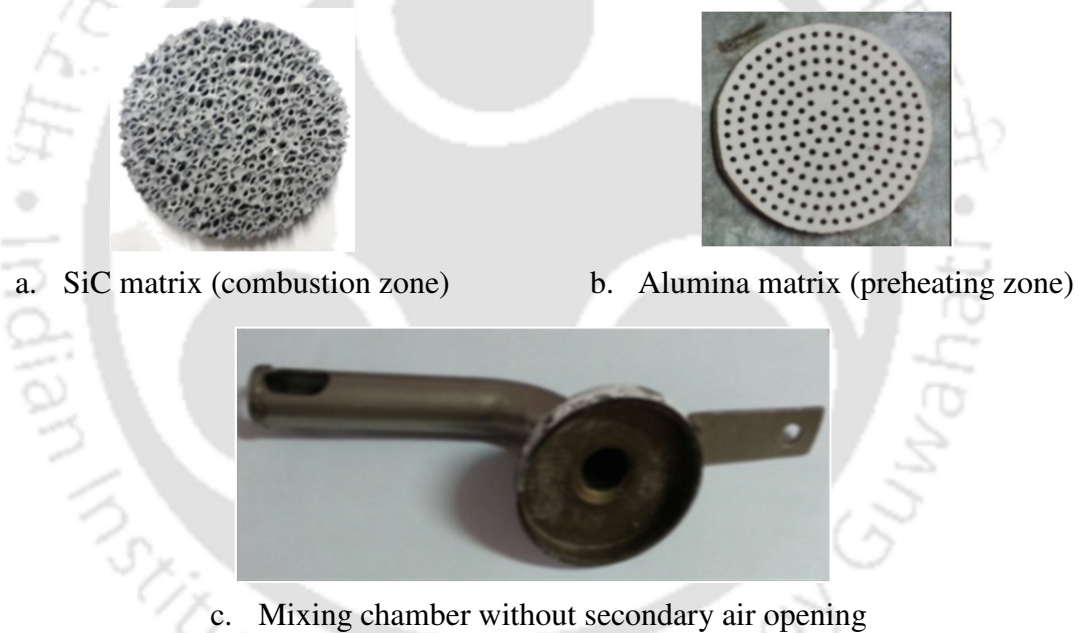
Fig.4.7. Two layer porous burner (a, b) and mixing chamber (c)
