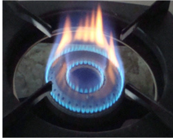
Fig. 4.2. Pictorial views of the free flame in conventional domestic cooking stove.
