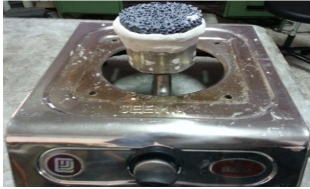
Fig. 4.13. PRB fitted on conventional stove with steel mixing chamber
