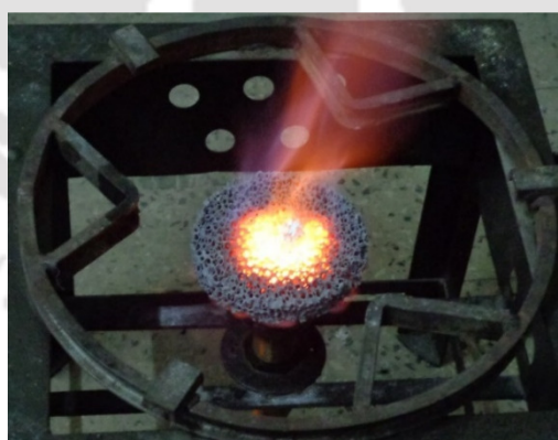
Fig. 5.2. Pictorial view of the SiC matrix as a burner in conventional stove
