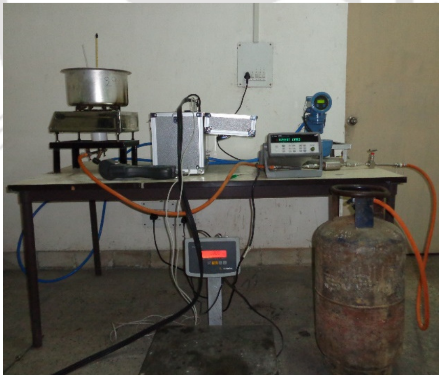
Fig. 4.18. Photographic view of experimental setup - for measuring emissions
