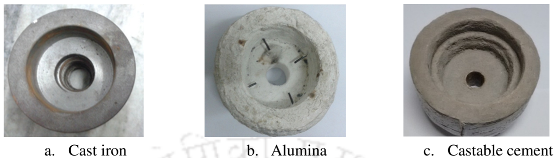
Fig. 4.15. Burner Casing of different materials
