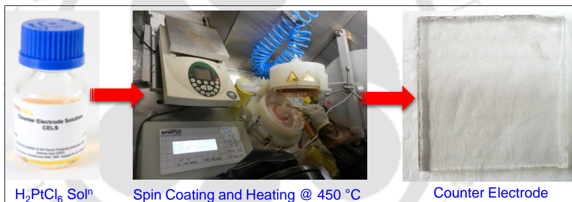
Figure 2.2.3 Pictorial presentation of step-by-step counter electrode preparation process.
