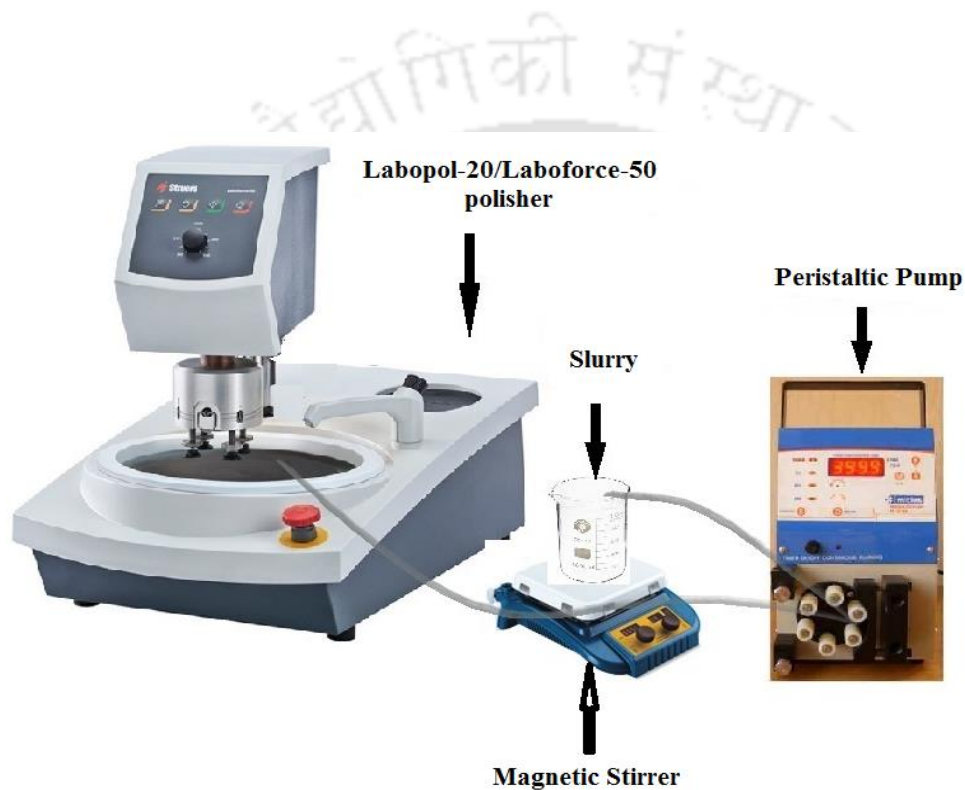
Figure 3. 1 Experimental Setup for CMP experiments
