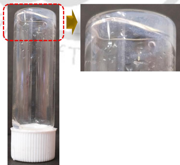
Figure A7.3: The minimum gelation concentration of GUA-IND required for gelation with (TBA)_2SO_4 .
