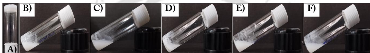
Figure A6.16: Gelation study of ADH-Py-m with CdCl 2 in different solvent mixtures viz. A) DMF-H 2 O, B) MeOH-H 2 O, C) EtOH-H 2 O, D) EA-H 2 O, E) ACN-H 2 O and F) THF-H 2 O.
