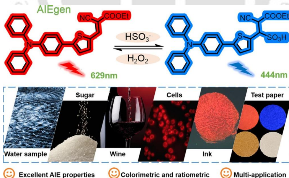
Figure 1.9: The structure of TPA-Y , recognition mechanism for \text{HSO}_3^-/\text{H}_2\text{O}_2 and applications of TPA-Y . (adapted from [1.29])
