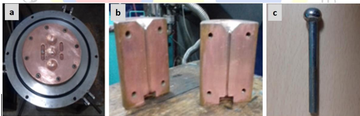
Figure 2.1 (a) Vacuum arc melting set up (b) Copper mould (c) Suction-cast (SC) sample
