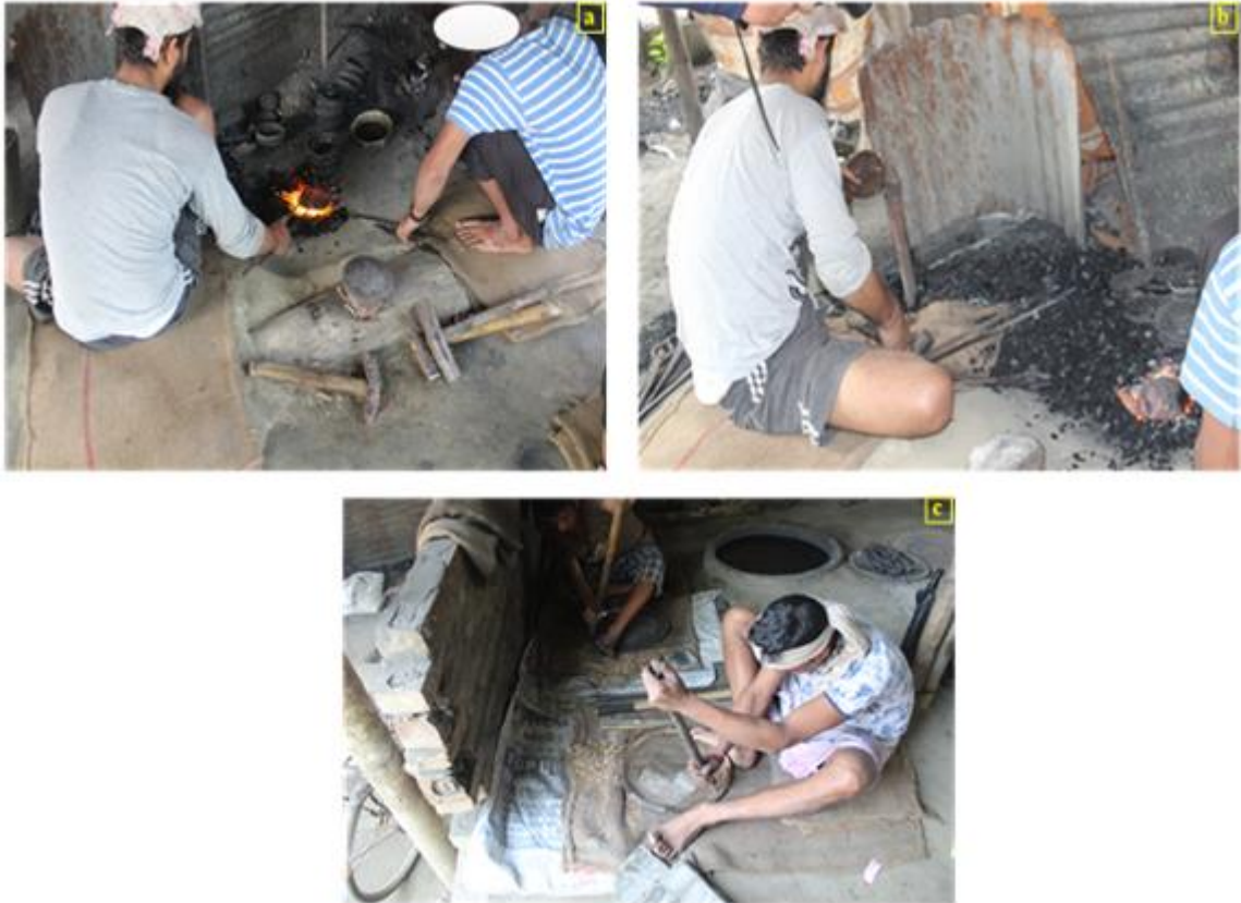
Figure 6.1 Different manufacturing techniques: a) Casting, b) Forging, c) Cleaning
