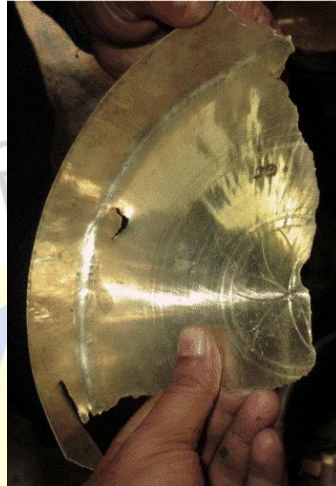
Figure 1.2 Failed bell metal products during cleaning
