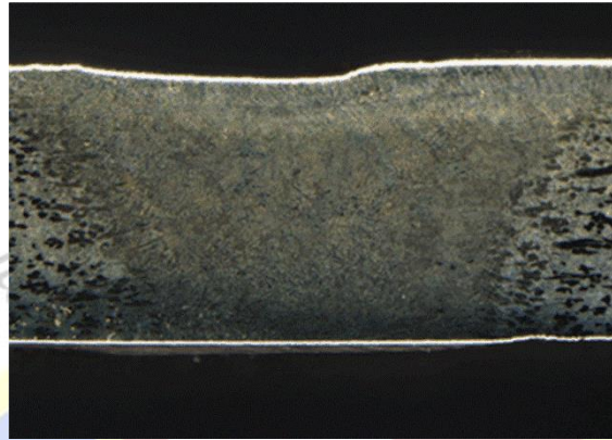
Figure 5.4 Cross-section of bell metal weldment at the knee point solution
