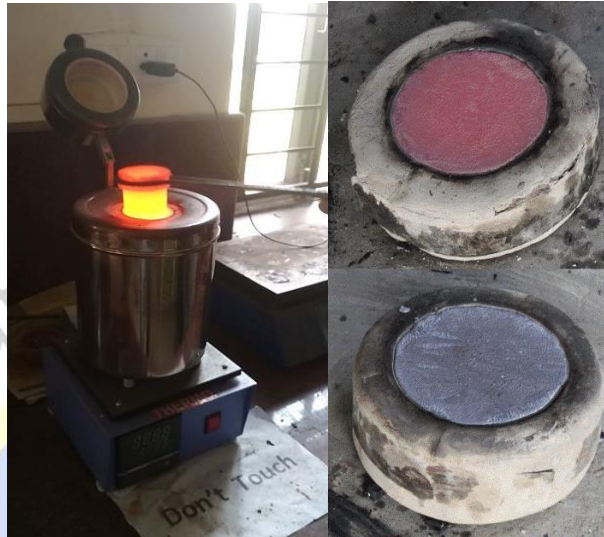
Figure 2.3 Casting: a) Furnace; b) Casted sample
