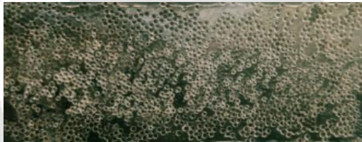
Figure 2. 2 Bead-based heterogeneous porous micromodel
