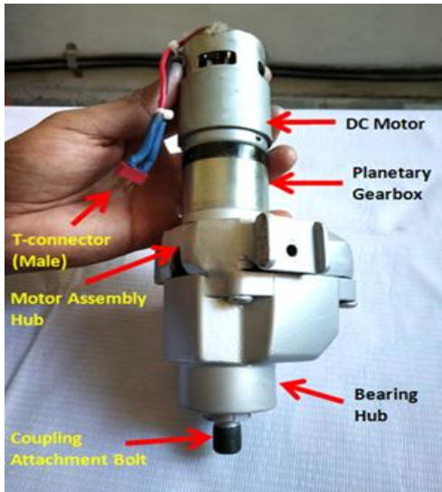
Fig. 4.14 Motor fixed to the hub
