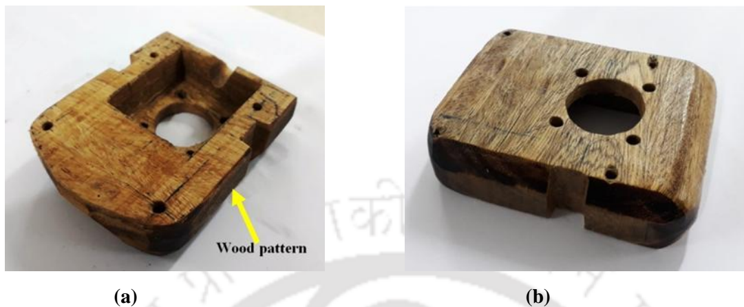
Fig. 4.5 The pattern of wood made for casting the block
