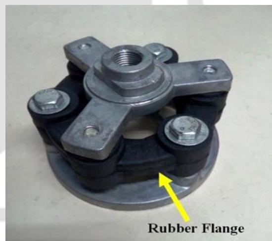
Fig. 4.14 Rubber flange inside the coupling
