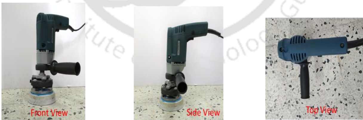
Fig. 4.1 .Image of the existing hand-held floor-polishing device
