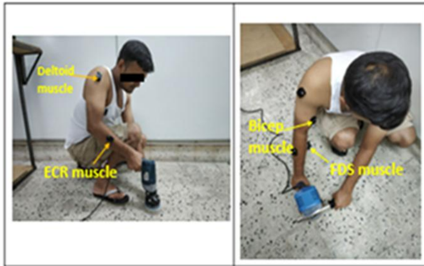
Fig. 3.3 Placement of electrodes on muscles
