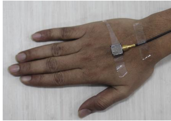
Fig. 3.4 Tri-axial accelerometer attached on the wrist of the operator during use of polishing machine (right-image)
