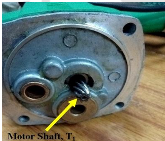
Fig. 4.8 The Motor shaft pinion of existing machine
