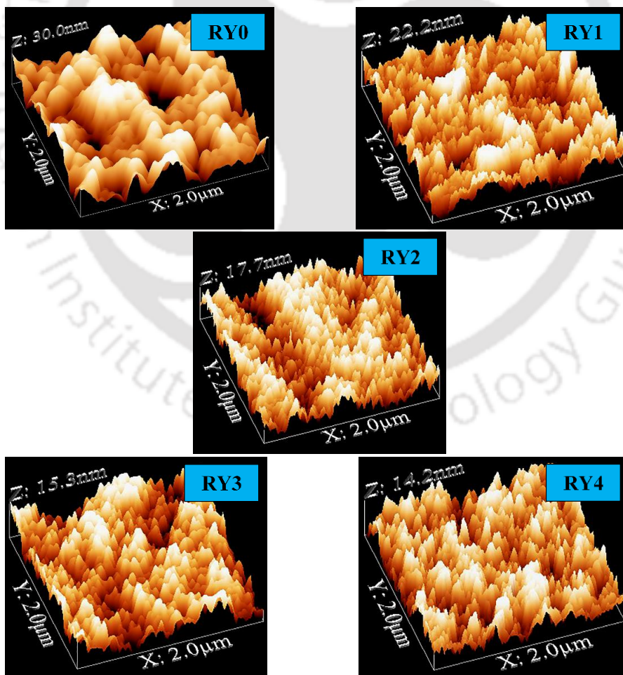
Figure 6.4. 3D AFM analysis of the membranes
