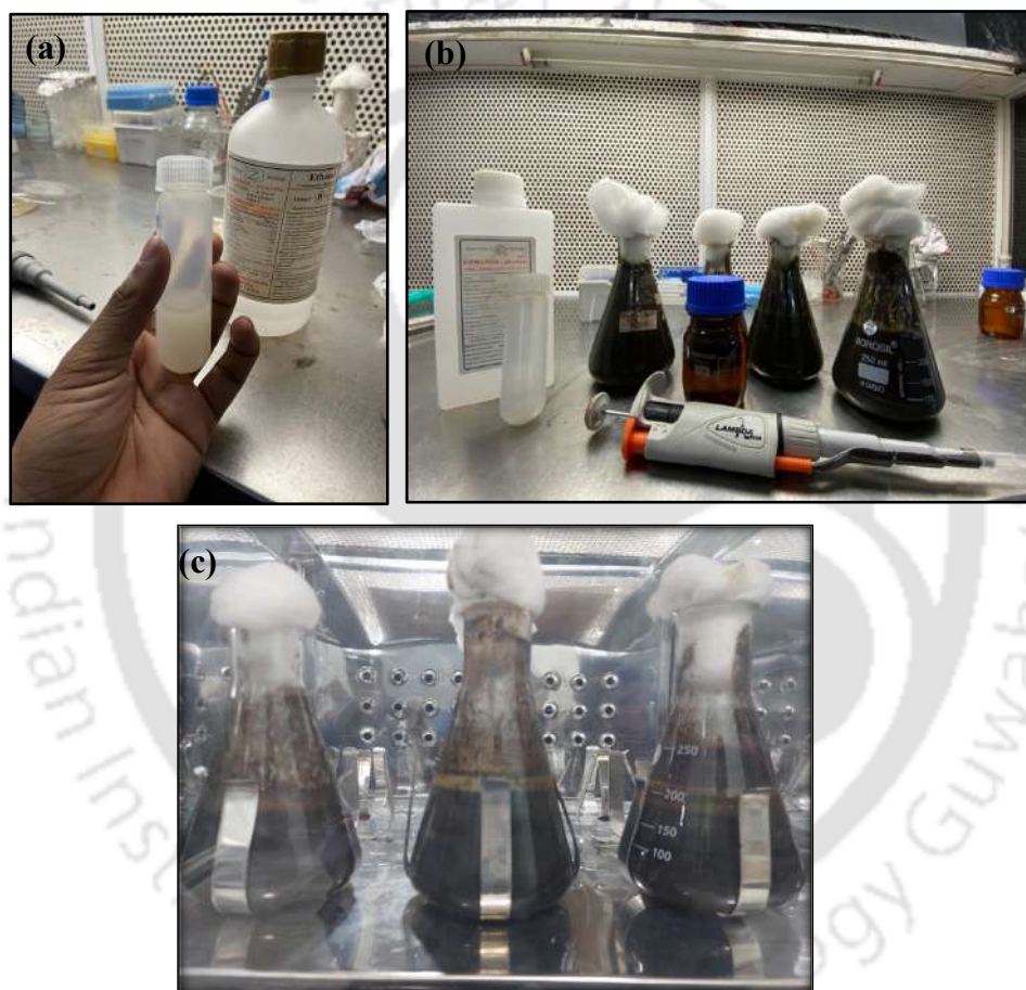
Fig. 3.5. (a) Bacterial inoculum, (b) samples inoculated with bacterial isolates at different dosages, and (c) incubation
