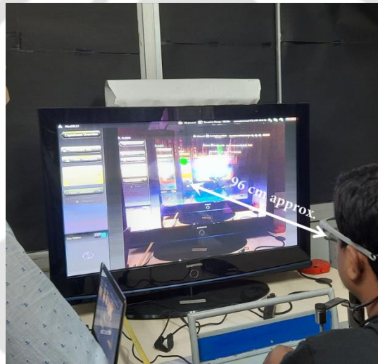
Figure 4. 5. Viewing distance of the stimuli (eye-tracking setup)
