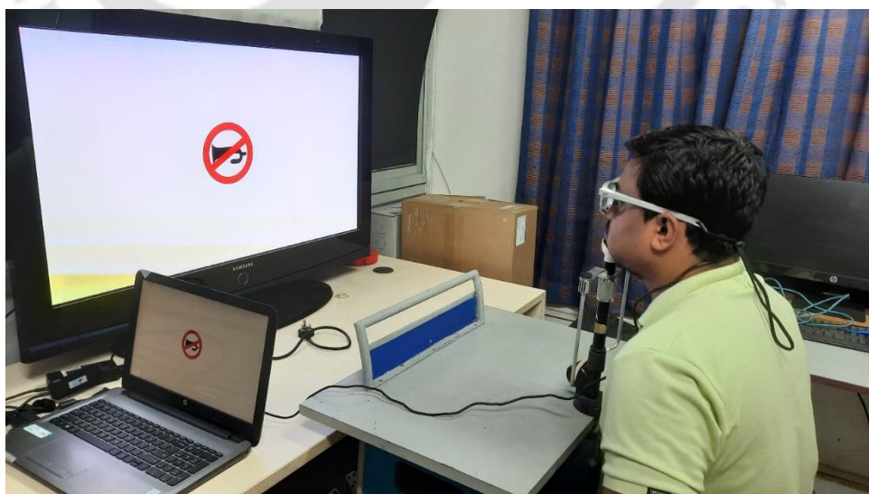
Figure A. 2. Eye experimental setup- big screen and laptop
