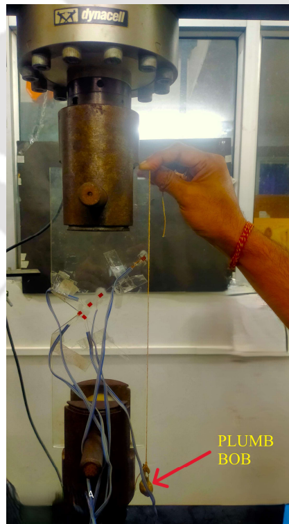
Figure 6.12 Checking of alignment of a specimen using a plumb bob.
