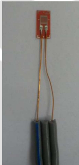
Figure 6.8 A typical 1 mm gage length, pre-wired TML strain gage.
