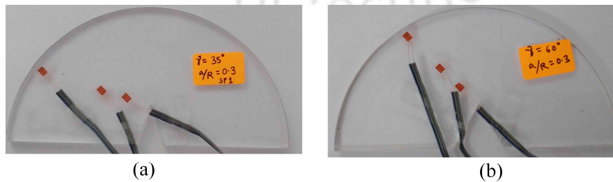
Figure 8.9 Three-point sharp V-notched SCB specimens employed in the experiments (a) \gamma = 35^\circ , a/R = 0.3 ; (b) \gamma = 60^\circ , a/R = 0.3 .
