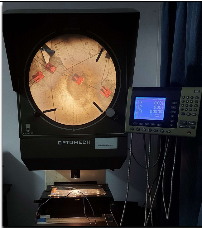
Figure 6.9 Optical profile projector for verification of orientation and location of a strain gage.
