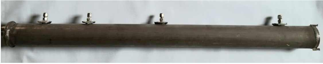
Fig. 6.1. (a) 3D sectional view of energy storage module (b) 2D sectional view of energy storage module with dimensions (thermocouple ports are not shown) and (c) photograph of the fabricated energy storage module
