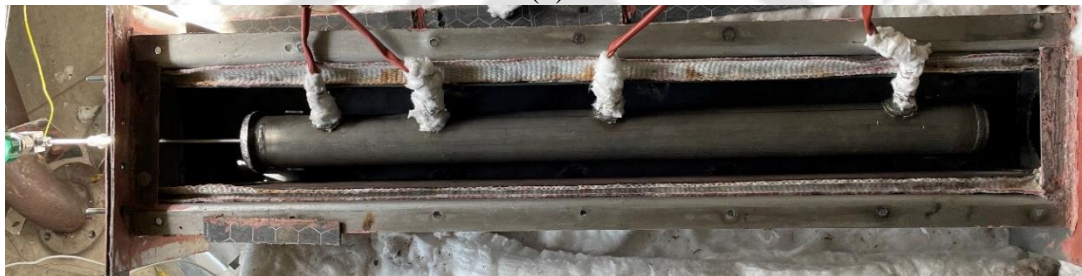
Fig. 6.4. Air calorimeter (a) 3D sectional view (right angle bend is not shown in the air outlet) (b) 2D sectional view (c) energy storage module placed inside the calorimeter
