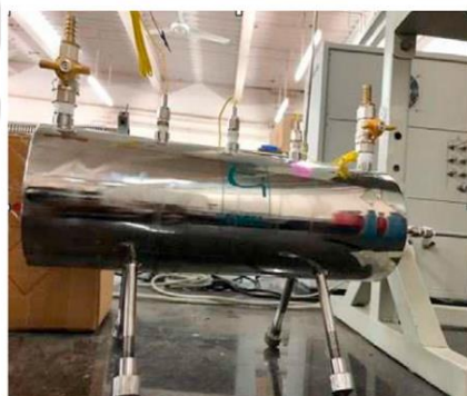
Embedded cooling tube reactor with an outer cooling jacket (Karmakar et al. 2021)
