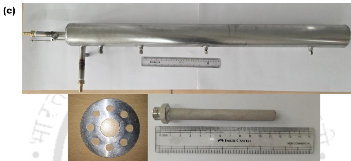
Fig. 5.1. (a) 3D sectional view and schematic of annular MH reactor with internal fins, (b) 2D sectional view of the annular MH reactor with internal fins with dimensions, and (c) pictorial view of the fabricated reactor, perforated aluminum fin, and sintered porous filter
