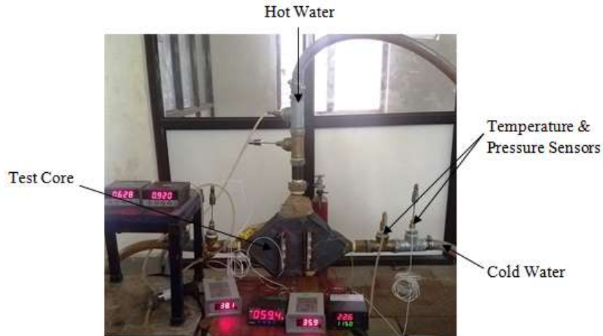
Fig. 3.34. Single-phase test setup
